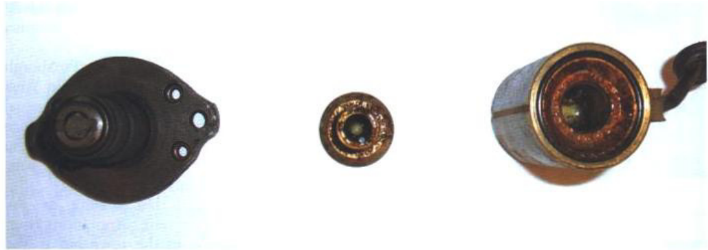
Before Quintolubric: A solenoid after 90 days use with previous fluid.
