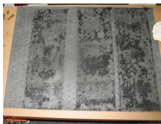
Absorbent after old rust preventive shows more damage
