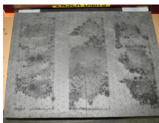
Absorbent after FERROCOTE® 5856 BF T1 shows less damage
