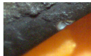
KTIP1550HPM at 60X, using previous coolant, after 9,600 holes in 1040V
