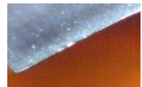
KTIP1550HPM at 60X, using QUAKERCOOL® 2776 after 13,500 holes in 1040V
