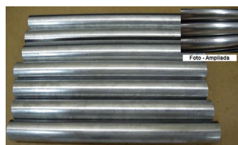
Wet galvanized pipes using FERROCOTE® 150 emulsion (10%). No white corrosion after 30 days.
