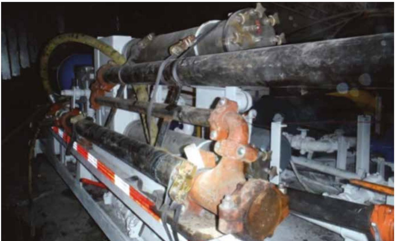
DUSTGRIP® JFP-95 manifold attached to a water car
