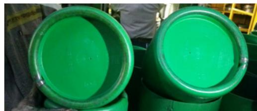
Performance comparison – Similar paint finish under press conditions with QUAKERCOAT® 856 GREEN (left) versus the solvent based coating (right)
