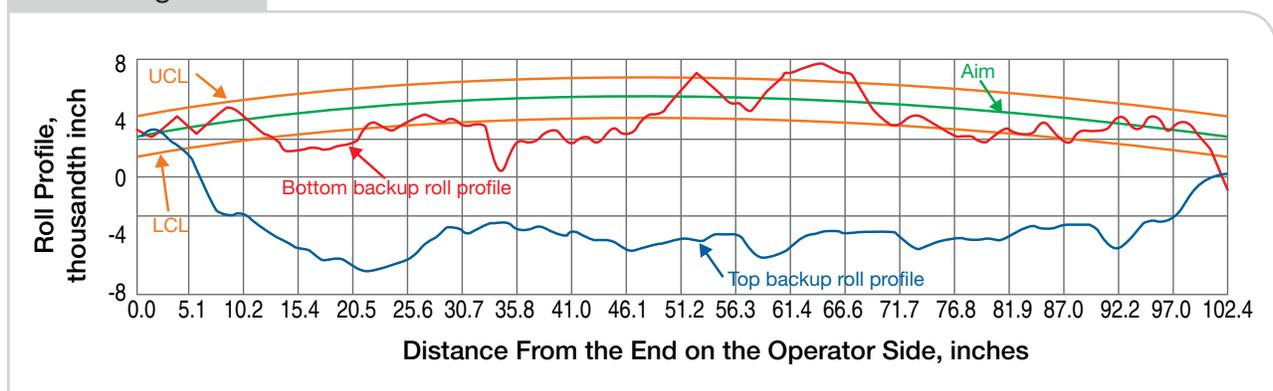
Profiles of the lubricated backup rolls after 9.99 million linear feet.
