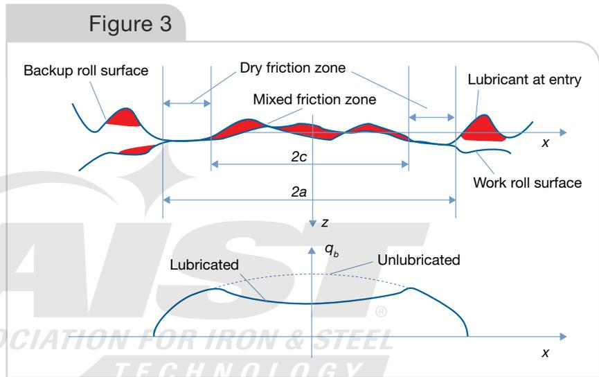
Dry friction and mixed friction in the contact zone.
