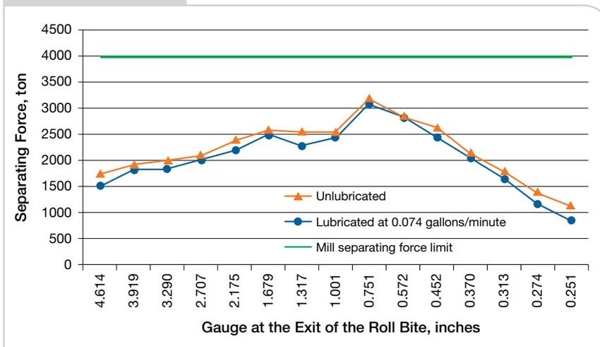
The effect of lubricant on separating force.
