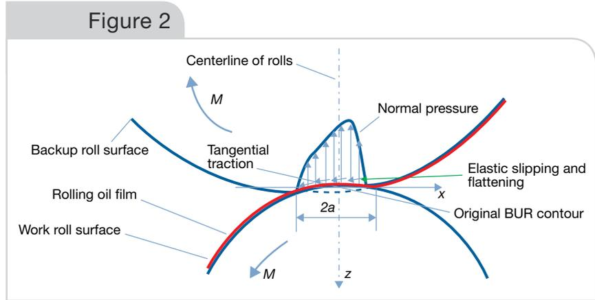
Normal pressure and tangential traction of the contact zone.
