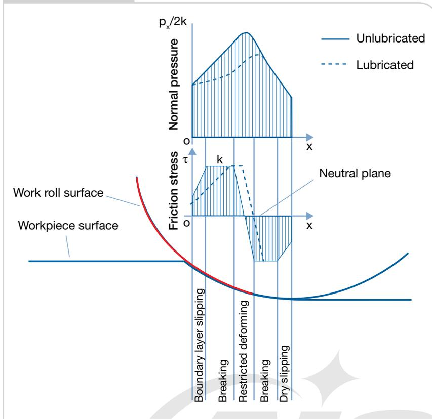
Friction stress and normal pressure in the roll bite.
