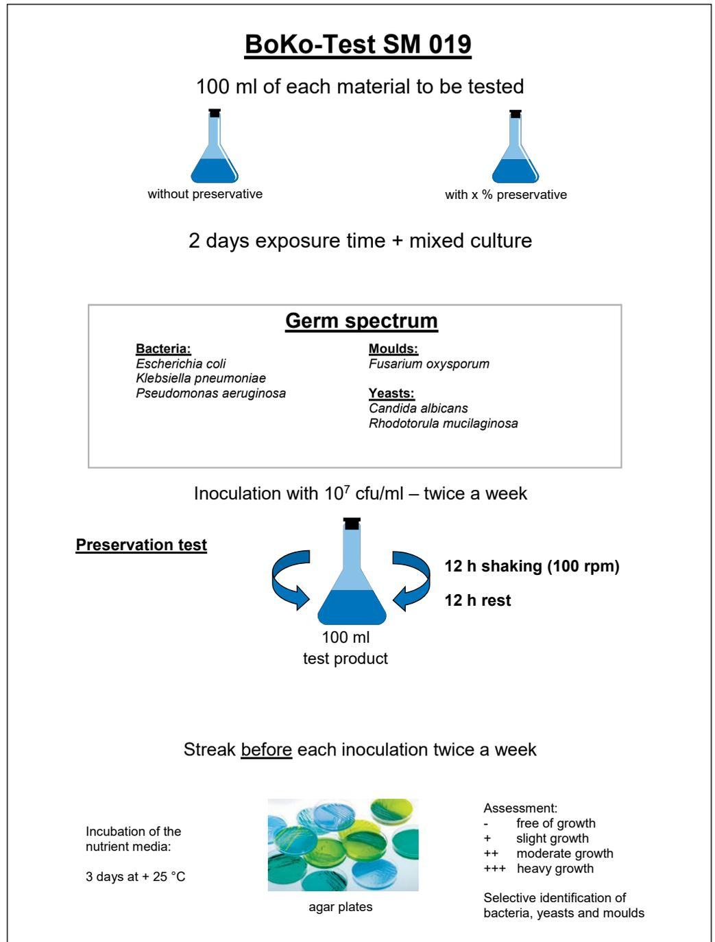
Figure 5. A procedure known as the BoKo-test is used to determine the bioresistance of a MWF. (Figure courtesy of Schülke & Mayr GmbH.)
