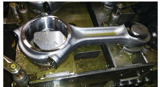
Image of the customer's connecting rod for a large engine positioned with fixtures on a deep hole drilling machine.
