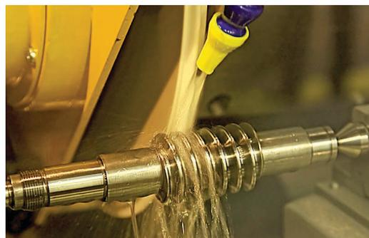
Worm Gear Grinding
