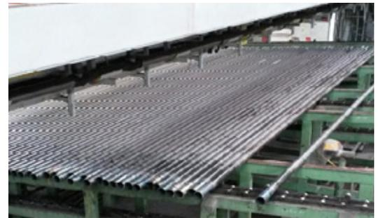
Oxide free pipes with the implementation of ADDITIVE CPN
