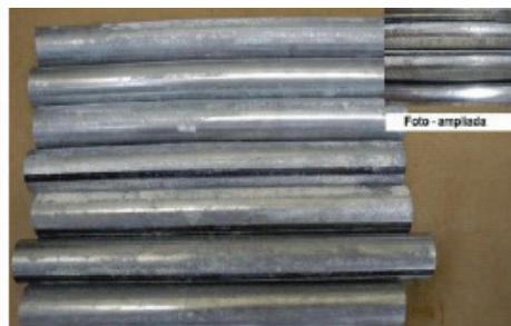
Wet galvanized pipes using the competitor's fluid emulsion (10%). Pipes completely corroded after 30 days.
